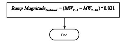
$(MW_{T-4} - MW_{T-60})$  represents the MW ramp of the generator resource/generator facility for a full minute prior to the event. The factor 0.821 adjusts this full minute ramp to represent the ramp the generator would have changed the system had it been allowed to continue on its ramp to T+46 unencumbered.
