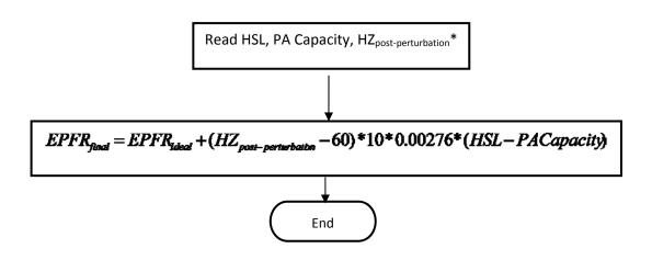
0.00276 is the MW/0.1 Hz change per MW of Capacity and represents the MW change in generator output due to the change in mass flow through the combustion turbine due to the speed change of the turbine during the post-perturbation measurement period. (This factor is based on empirical data from a major 2003 event as measured on multiple combustion turbines in ERCOT.)
